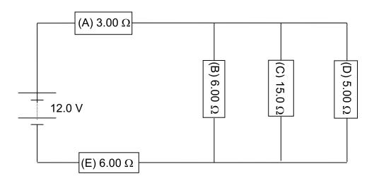
(a) Without doing any calculations, explain which of the two 6.00  $\Omega$  resistors (B or E) must have the larger potential difference across it. (3 marks)
