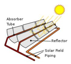
absorber tube. However, seasonal changes in the angle of sunlight parallel to the trough does not require adjustment of the mirrors, since the light is simply concentrated elsewhere on the absorber tube. The absorber tube may be enclosed in a glass vacuum chamber, as the vacuum significantly reduces convective heat loss.
